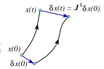
**Figure 1.10:** The Jacobian matrix J' maps an infinitesimal displacement  $\delta x$  at  $x_0$  into a displacement  $J'(x_0)\delta x$  finite time t later.
