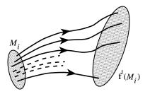
**Figure 2.2:** The evolution rule  $f^t$  can be used to map a region  $\mathcal{M}_i$  of the state space into the region  $f^t(\mathcal{M}_i)$ .
