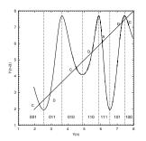
$y_{k+3} = P_1^3(y_k, z_k)$ , the third iterate of Poincaré return map is used to pick starting guesses for the Newton-Raphson searches for the two 3-cycles:
