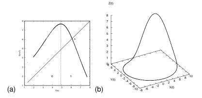
(a)  $y \rightarrow P_1(y, z)$  return map for x = 0, y > 0 Poincaré section (b) the  $\overline{1}$ -cycle found by Newton-Raphson, taking the fixed point  $y_{k+n} = y_k$  as initial guess (0, y(0), 0)
