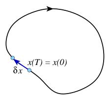
hence a longitudinal displacement  $\delta x = v(x_0)\delta t$  is mapped into itself by the cycle Jacobian matrix  $J_p$ .
