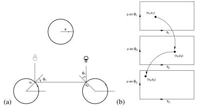
**Figure 15.15:** (a) Poincaré section coordinates for the 3-disk game of pinball. (b) Collision sequence  $(s_1, p_1) \mapsto (s_2, p_2) \mapsto (s_3, p_3)$  from the boundary of a disk to the boundary of the next disk presented in the Poincaré section coordinates, and coded by the return maps sequence  $P_{3 \leftarrow 2} P_{2 \leftarrow 1}$ .
