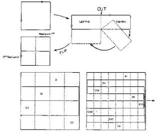
FN3-4. Iterative construction of the symbol plane.
