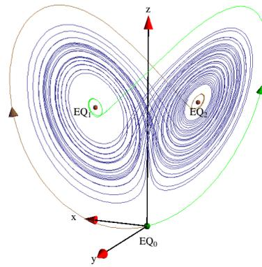
**Figure 9.3:** Lorenz attractor of figure 3.7, the full state space coordinates  $[x, y, z]$ , with the unstable manifold orbits  $W^u(EQ_0)$ . (Green) is a continuation of the unstable  $e^{(1)}$  of  $EQ_0$ , and (brown) is its  $\pi$ -rotated symmetric partner. Compare with figure 9.4. (E. Siminos)
